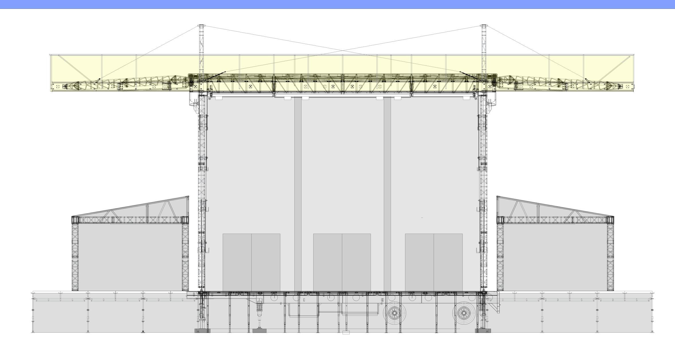
**TOTAL WEIGHT CAPACITY OF ROOF STRUCTURE: 97,600 LBS**
