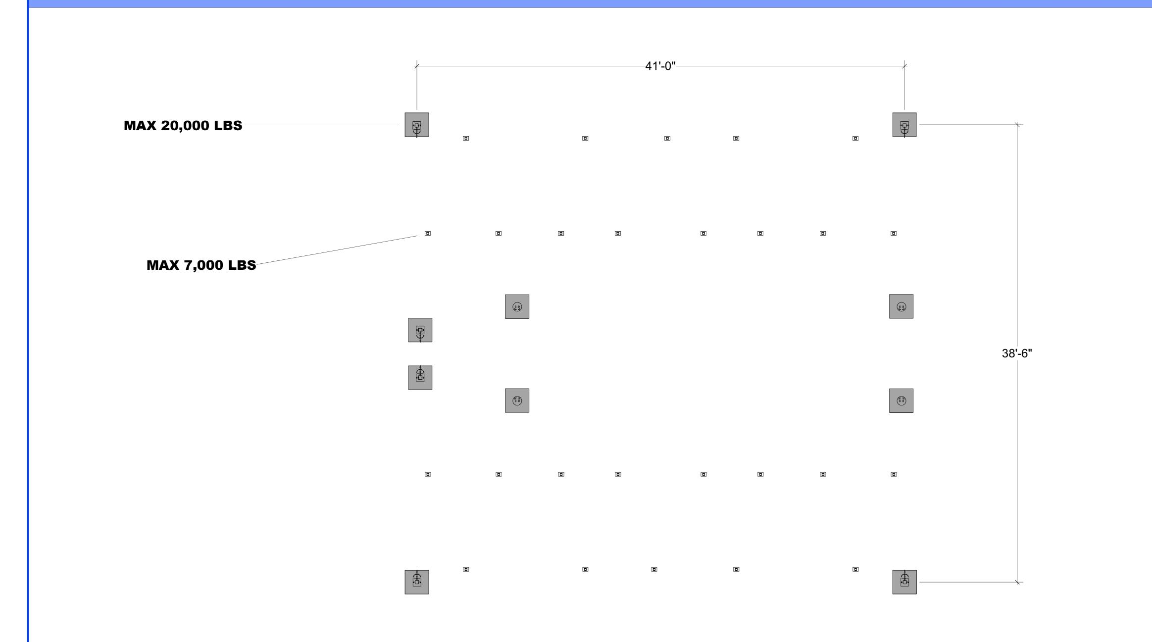
SHOWN IS MAX WEIGHTS ALLOWABLE AS PER ENGINEERING TOTAL GROSS WEIGHT OF STRUCTURE IS 56,000 LBS TO BE SPREAD OUT ON POINTS SHOWN ADDITIONAL WEIGHT WOULD BE DETERMINED WHEN PRODUCTION FIGURES ARE ADDED IN.
